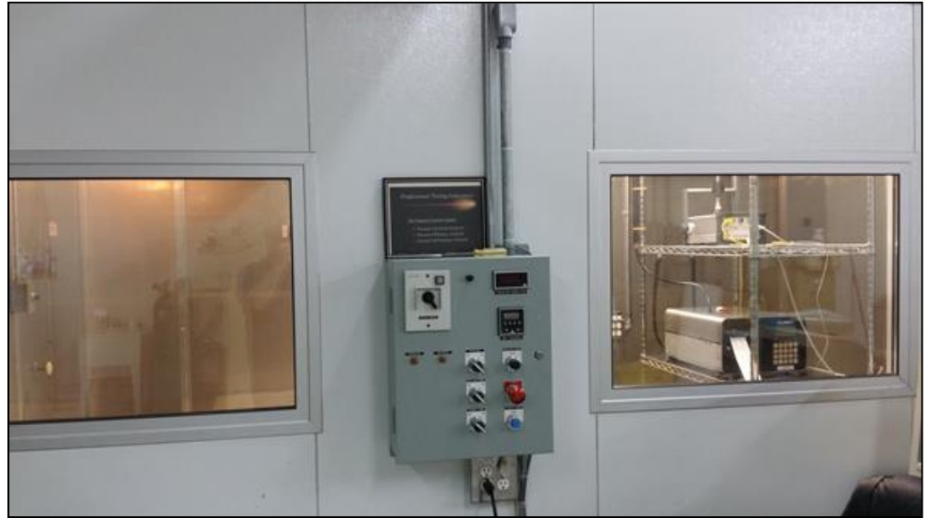
ASTM E1333 Standard Test method for Determining Formaldehyde Concentrations in Air and Emissions Rates from Wood Products using a Large Chamber
